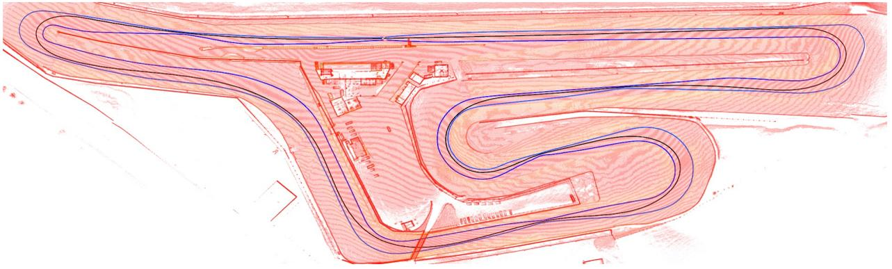
Fig. 2. Circuit de Croix-en-Ternois in France. Point cloud data are red. Track borders are blue and the racing line is black.
